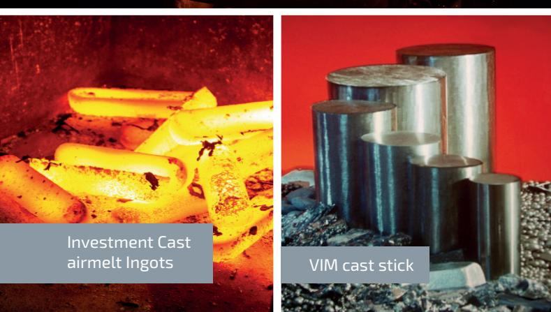
By using high-frequency Airmelt Induction Furnaces, William Rowland can produce uniform cast ingots from 500kg – batches upward. Additionally, for material where lower gas content is required, we can melt and cast under vacuum (VIM) with batch sizes 2000kgs and upward in a variety of diameters. Both processes are overseen by our metallists and the latest analytical control techniques, such as Spectro analysis and ICP-OES.
